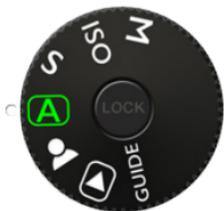
The **Mode** dial selects the mode of operation. M: fully manual, ISO: ISO-priority, S: shutter-priority, A: automatic. Also access to the front camera (if available), Review/Share view, GUIDE, which opens up this User Guide. For more on 645 PRO Mk III's shooting modes, see page 14. To see how the Mode dial may be configured, see page 42. (TIPS: double-tapping the Mode dial provides a quick shortcut to the Review/Share view; a long press locks it.)
